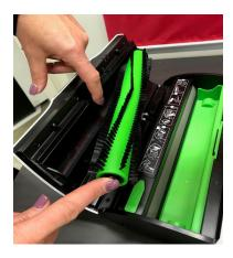
(3) Clean behind the polymer cleaning roller at least twice a week, by wiping the sink/drain (metal grate) with a paper towel. (very important) Hair, dirt etc will accumulate here.
