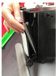
Once you have removed the sink drain (chrome grate), clean inside the channel, pictured on the LEFT, with a paper towel. When reinstalling the sink drain make sure that it is reinstalled the correct way. The "high side" or "lip side" of the sink drain should face the opening with the cleaning roller motor at the low side. See image 2 & 3 below:
