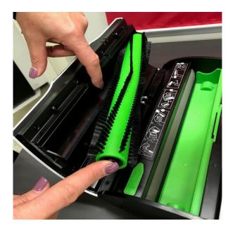
3 Clean behind the polymer cleaning roller at least twice a week, by wiping the sink/drain (chrome grate) with a paper towel. (very important) Hair, dirt etc will accumulate here.
