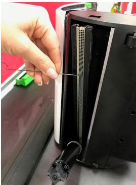
6 Once you have removed the sink drain chrome grate, clean inside the channel, pictured on the LEFT, with a paper towel. When reinstalling the sink drain make sure the foam filter is in place, see image on the right. The sink drain can only fit in one way, the lip side of the drain must face the opening.
