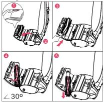
3 Insert a new brush roller, close the cover after it is well assembled.
