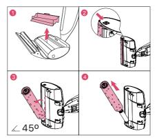
Insert a new cleaning roller onto the motor, push and fix it into the cleaning head till the lateral button in place.
