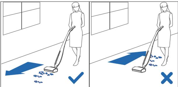
2. To avoid inefficient cleaning, the cleaning path shown in the following pictures is recommended.
